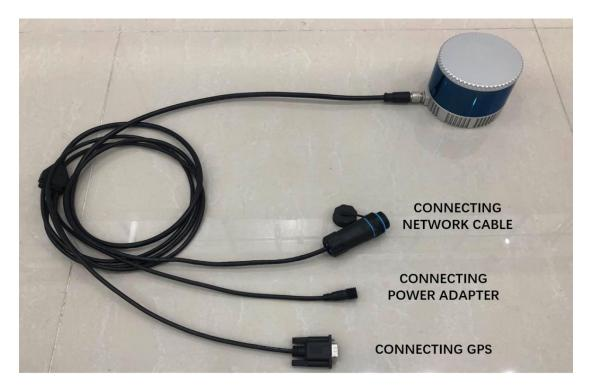
Figure 3.1 Connecting Lidar and Computer
