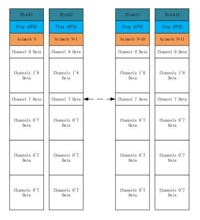
The data block structure of the C1 single echo packet is as follows:
