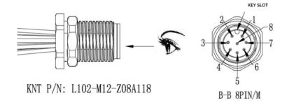
Figure 2.1 Cable Connector on the Lidar Base
