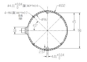
Figure 1.4 C1 Lidar Base (unit: mm)
