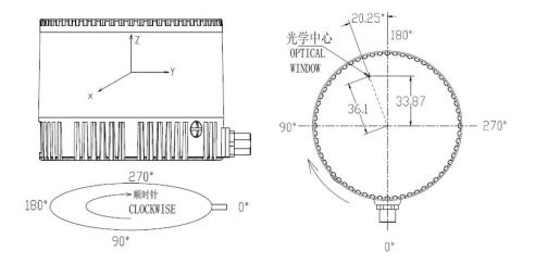
Figure 1.2 Coordinates & Scanning Direction
